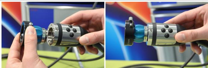
TV-Adapter connection to an endoscope
